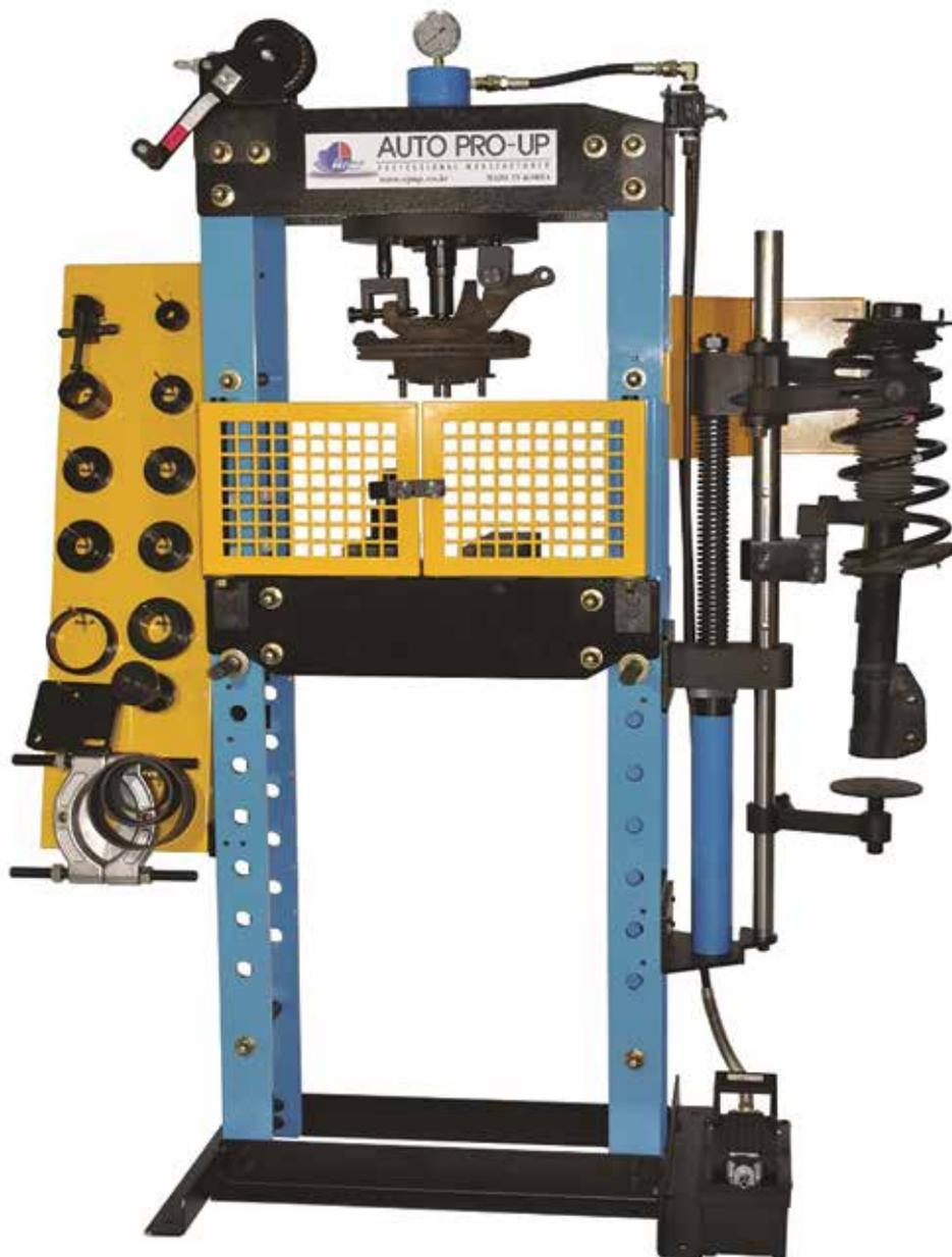
**T**he PS-2000 has been designed and manufactured in Korea specifically for the needs and requirements of the automotive repairer. With a 30-tonne rating operated by a conveniently located foot pedal, the *Air Over Hydraulic Pump*, the PS-2000 performs all the needs faced on a
