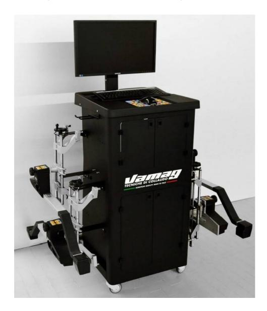
Model: am-2003-T. Bluetooth 8 sensor CCD wheel aligner for trucks, bus, trailers, semi-trailers, and rear-steering vehicles. With patented 3 point clamps (13" to 30", no need run-out compensation or standard 4 point clamps (13" to 25".
